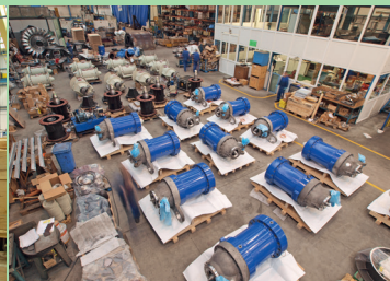
Fabrication and finish assembly injectors ready for erection
