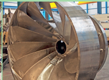
Francis runners fabricated in forge and welding process in three parts
