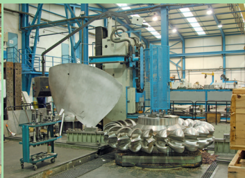
Machining process of Kaplan blade and finish Pelton runner different dimensions till 4,5 diameter
